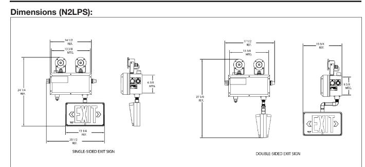
EXS, EXD Option – N2LPS LED Light-Pak<sup>™</sup> with Optional Emergency Exit Luminaire
